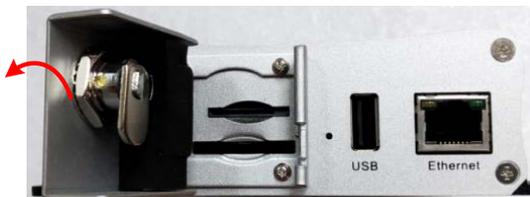
3. Lock the card protection plate using the supplied Card Lock Key.
