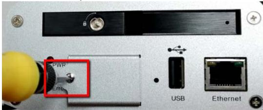
2. Lift up the card protection plate and insert a 3G/4G SIM card into the Card slot (the upper one).
