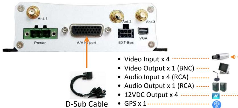
**Camera Connection:** Connect to the eZ.HD cameras using the four Video Input cables. To supply power to cameras, connect the 12VDC Output cables (500mA each) to the cameras. Note that the mobile DVR doesn't support HD-TVI / HD-CVI / HD-SDI cameras.
