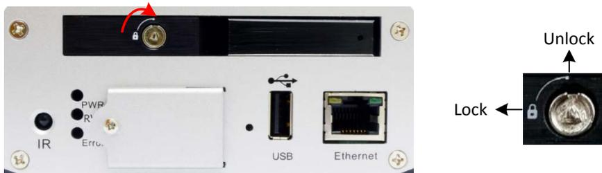
2. To install the SSD, pull the Release Latch to open the SSD Tray Arm.
