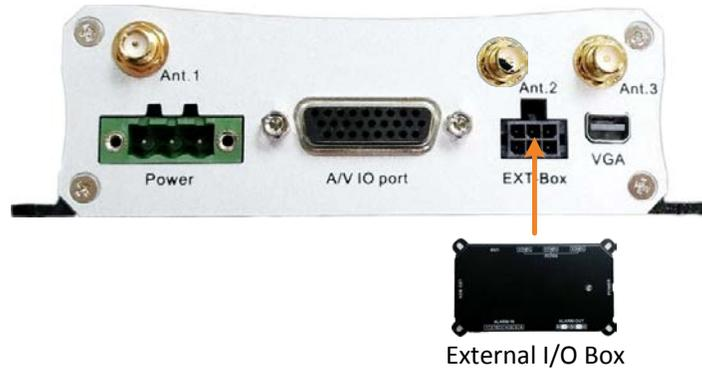
If you want to monitor mobile DVR status, such as storage, GPS, 3G/4G/WiFi connectivity; or trigger alarm among the mobile DVR, Control Center (Genie XMS / Xfleet) and External I/O Box, you can optionally connect the LED Indicates Box to the External I/O Box. Note that the LED Indicates Box must work in conjunction with External I/O Box. For more details about the LED Indicates Box, please refer to the *User's Manual of LED Indicates Box*.
