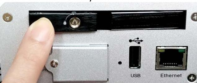
5. Lock the SSD Tray using the supplied SSD Lock Key.
