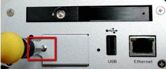
2. Lift up the card protection plate and insert a SD card into the SD Card slot (the lower one).
