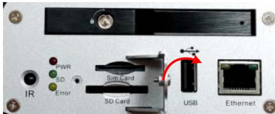
3. Screw back the card protection plate. The SD card installation is now complete.
